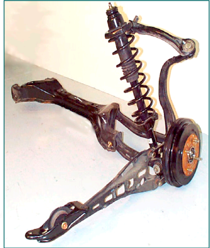
Example of a Double Wishbone Rear Suspension System
