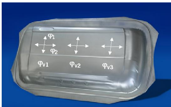
Figure 28: Circle Grid Placement – Sheet Hydroforming
