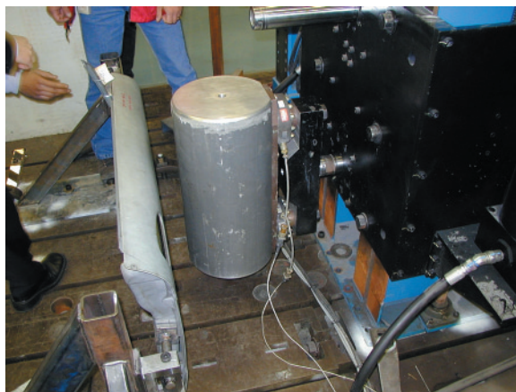
Figure 40: Quasi-Static Intrusion Test Set Up
