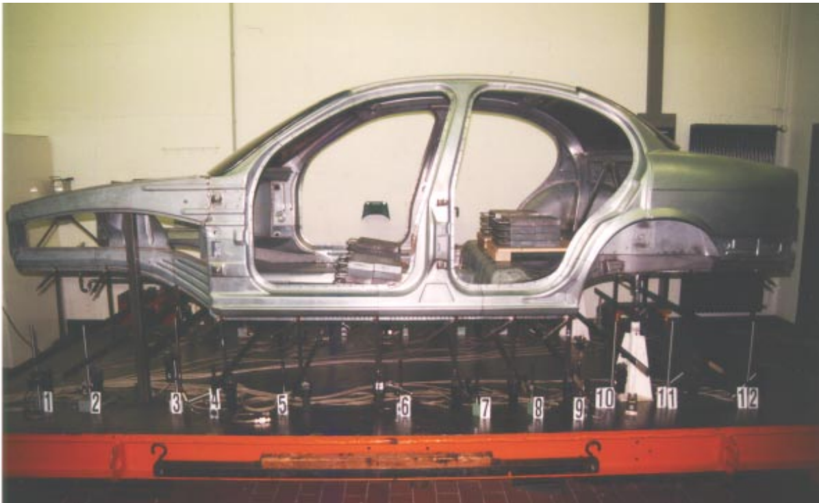
Figure 10.3.2.2-1 DH on Test Rig for Static Bending
