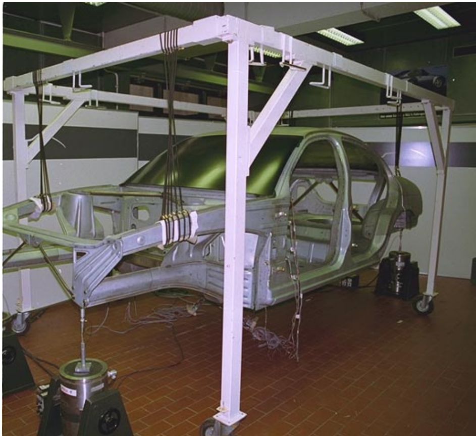
Figure 10.4.2-1 DH on Test Rig for Modal Analysis
