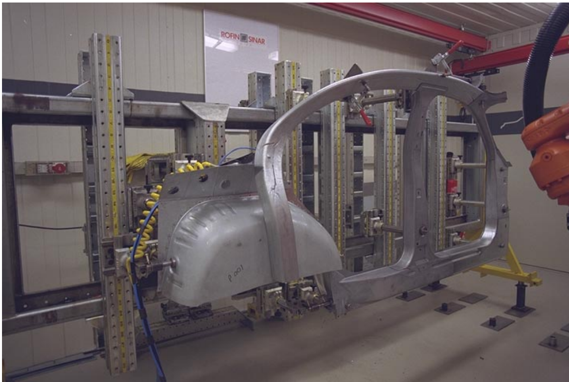
Figure 9.3-3 Assembly Fixture - Bodyside Inner Subassembly
