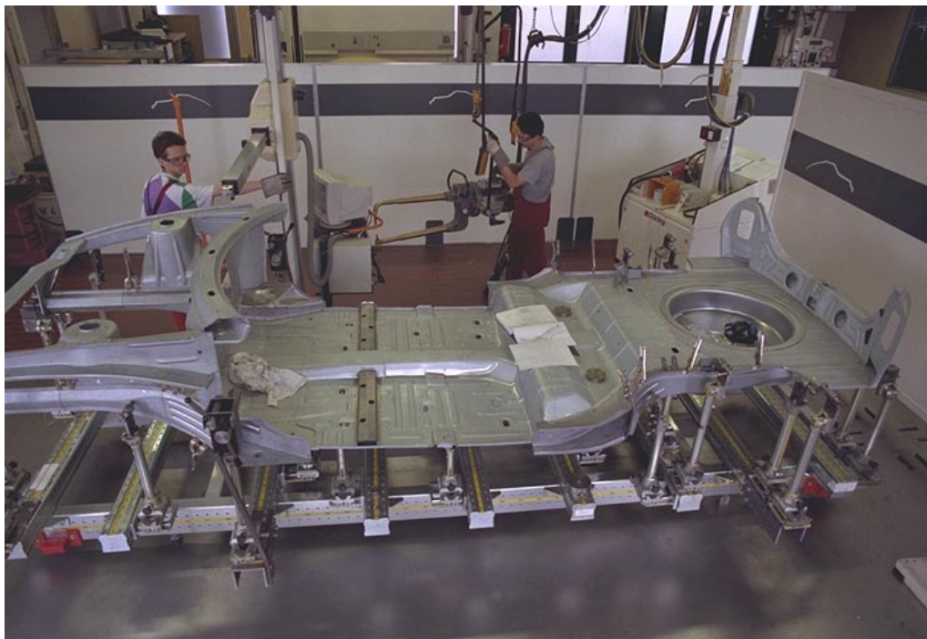
Figure 9.5.2-3 Subassembly Underbody Complete
