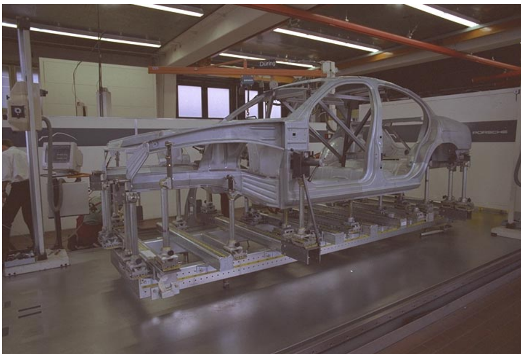
Figure 9.5.2-7 Sub-Assembly Body Side Outer, with Body Side Inner and Underbody
