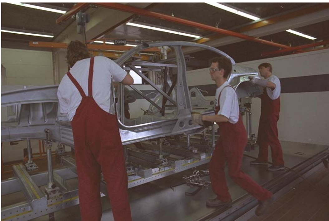
Figure 9.5.2-5 Assembly Body Side Inner to Underbody
