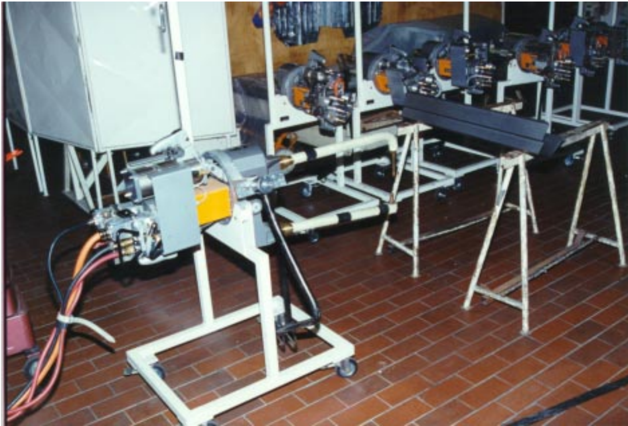
Figure 9.5.1-3 Weld Gun Station
