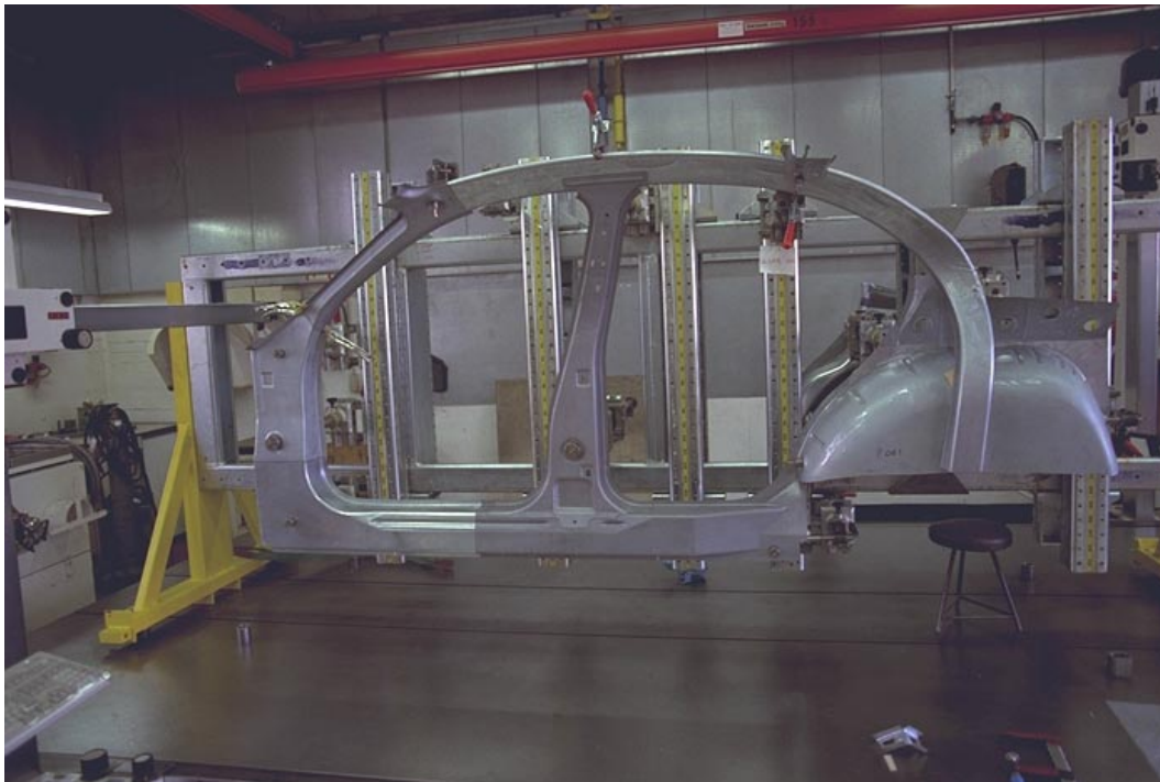
Figure 9.5.2-4 Subassembly Body Side Inner
