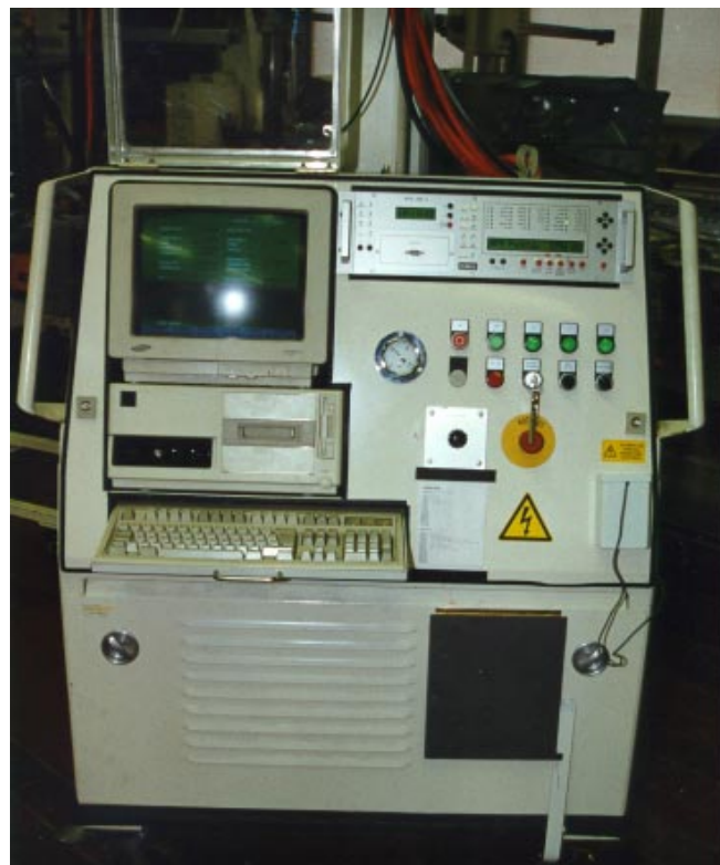
Figure 9.2.2-3 Medium Frequency Spot Welding Equipment
