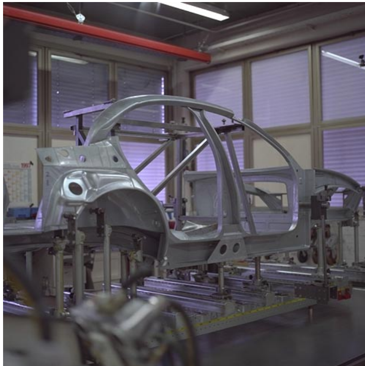
Figure 9.5.2-6 Subassembly Body Side Inner with Underbody
