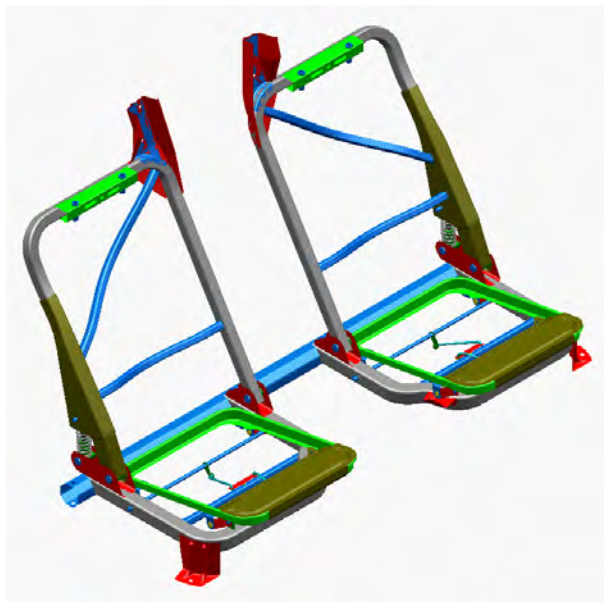
Figure 12.1.1-2 Front seat structure assembly
