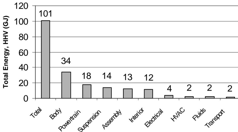
**Figure 8. ULSAB-AVC PNGV-Gas Engine Vehicle Production Energy by Subsystem, Assembly and Transport.**
