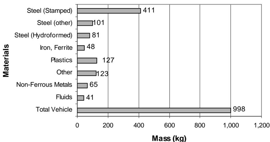
**Figure ES-3. Material Distribution for the ULSAB-AVC PNGV-Gas Engine Vehicle.**
