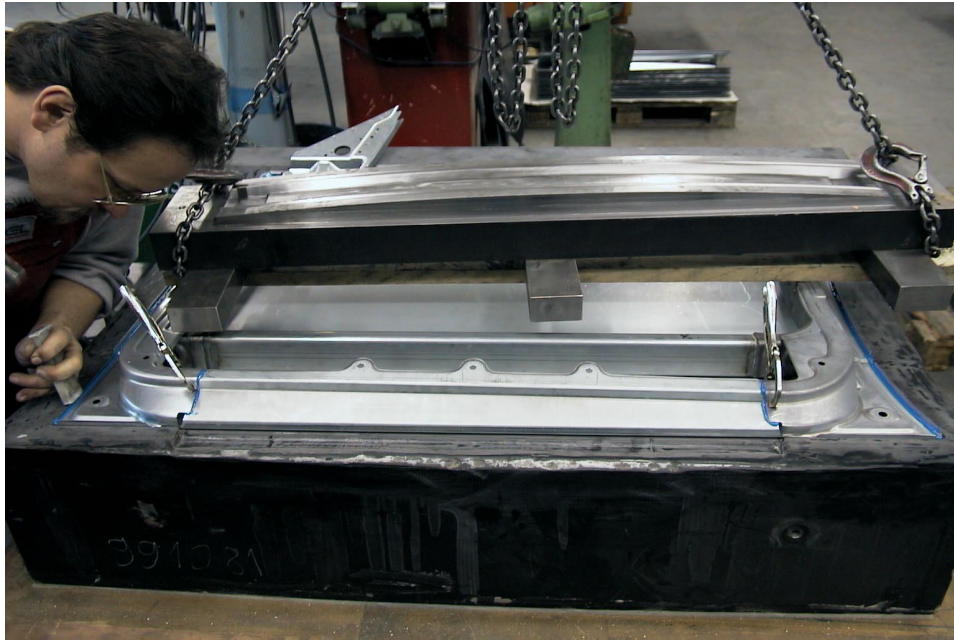
Figure 9.3-6 Subassembly #3: Bonding and hem flanging of the Front Door Outer
