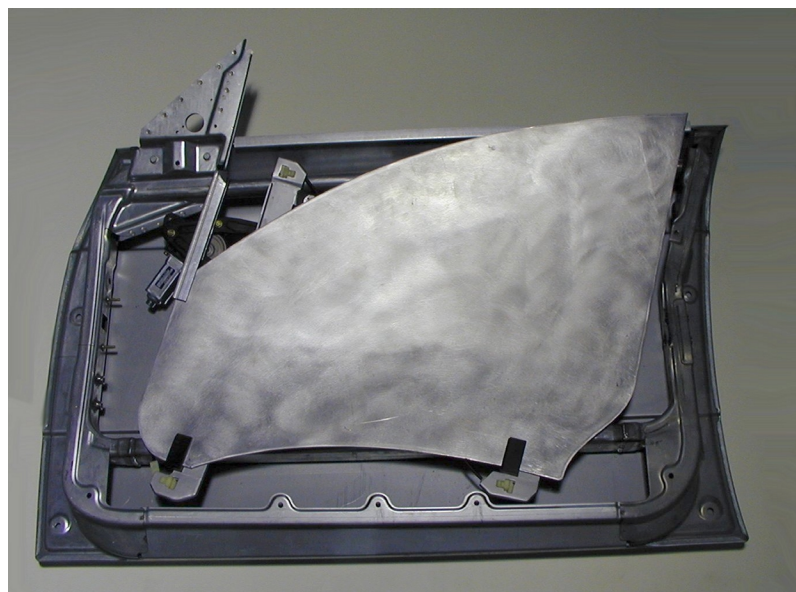
Figure 3.2.2-2 Subassembly #2 - door structure complete with window regulator & glass
