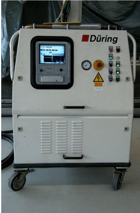
Figure 9.1.2-1 Düring™ weld device with Matuschek™ control system
