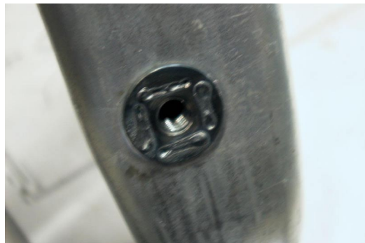
Front Door Hinge Bushing to Front Door Hinge Tube (#1)
