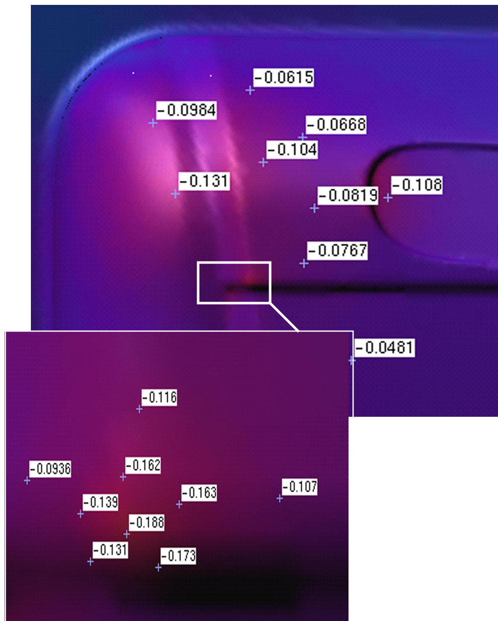
Figure 7.3.4-3 Panel Front Door Outer upper left corner thinning
