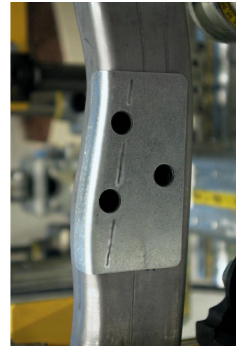
Reinforcement Latch to Front Door Latch Tube (#3)
