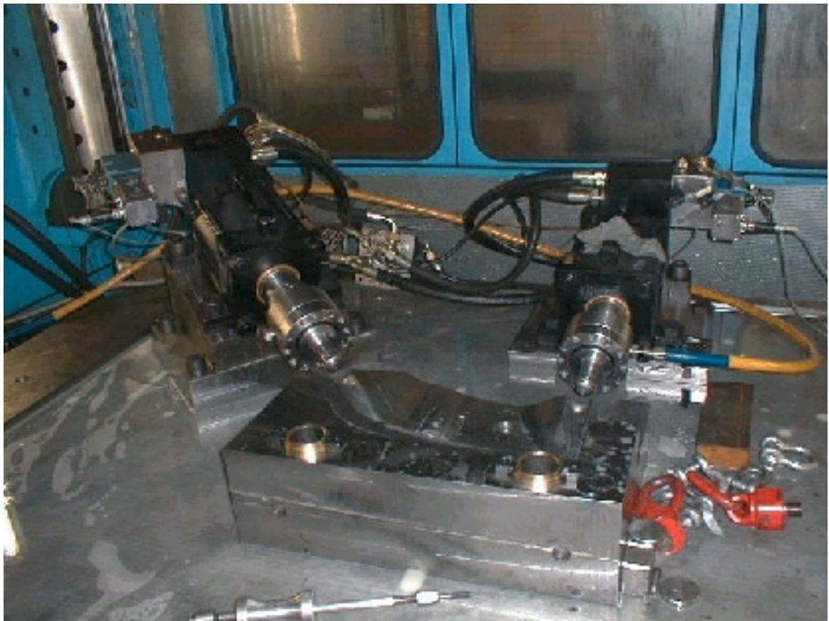
Fig 6.6.3.1-4 Hydroforming tool
