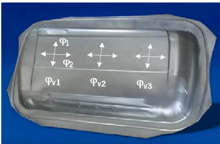
Figure 4.4.1-1 Circle Grid Placement
