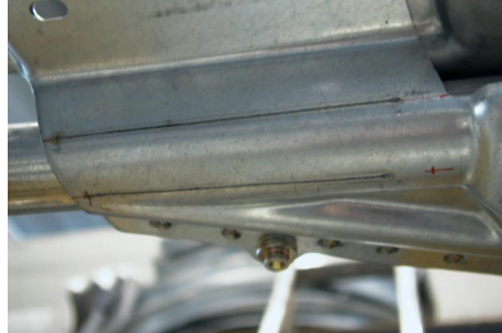
Mirror Flag Outer to Front Door Outer Belt Reinforcement (#6)
