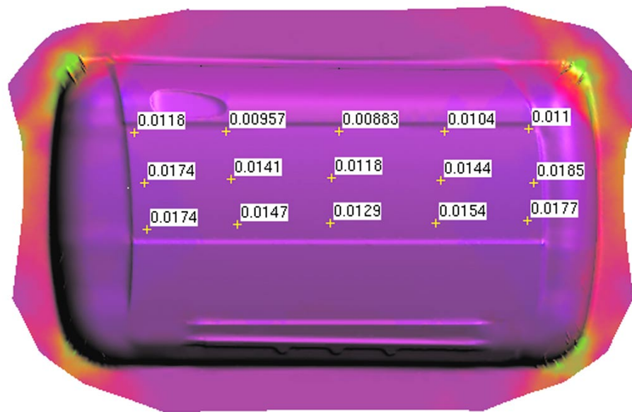
Figure 3.2.1-2 Minor Strain of the Panel Front Door Outer (DP600 0.6mm)
