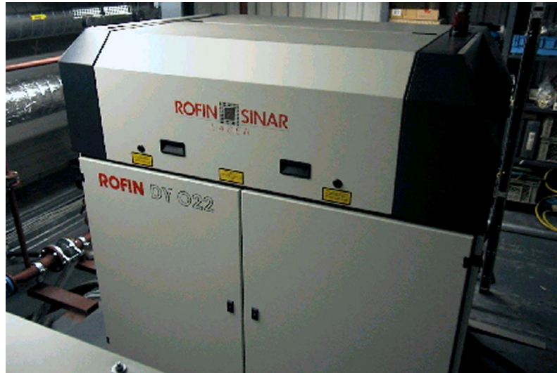
Figure 9.1.1-1 New diode pumped solid state laser of Rofin Sinar
