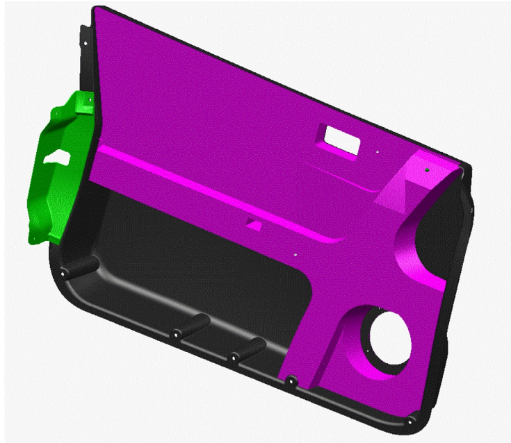
Figure 3.1.1.5.1-2 Trim panel with inner foam structure
