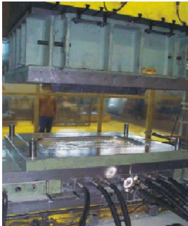
Figure 4.2.4-1 AHM door panel forming tool
