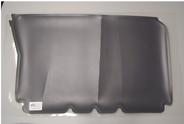
Figure 3.1.1.5.2-6 Frontdoor vapor barrier
