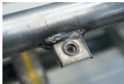
Regulator Attachment to Front Door Outer Belt Reinforcement
