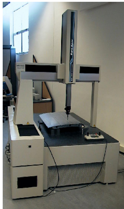
Fig. 10.3.3-2 Mitutoyo 3D measuring machine
