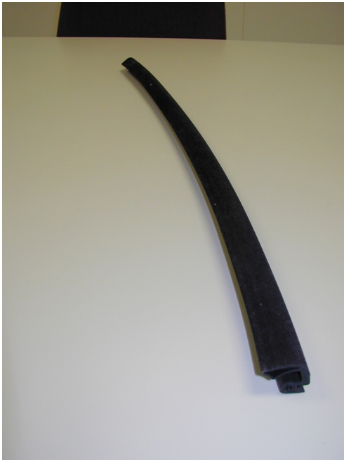
Figure 3.1.1.5.2-4 Front door inner belt seal
