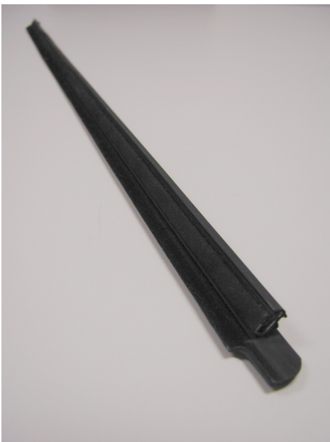
Figure 3.1.1.7-2 Front door outer belt seal
