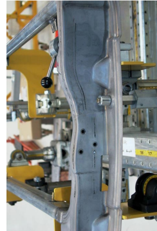
Front Door Inner Rear to Front Door Latch Tube (#5)
