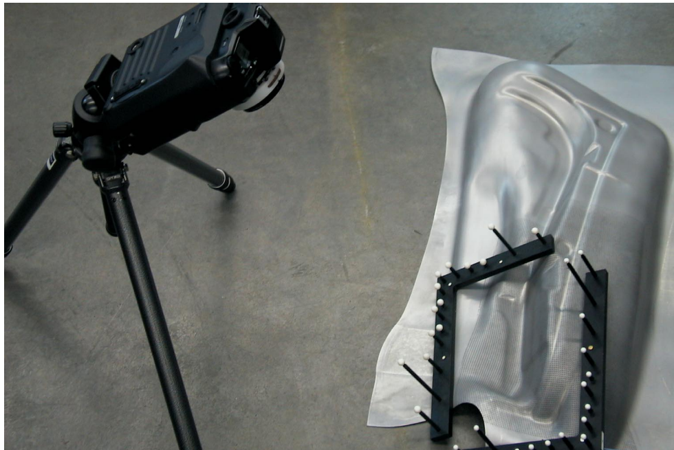
Figure 8.4.1-3 Circle grid strain measurement
