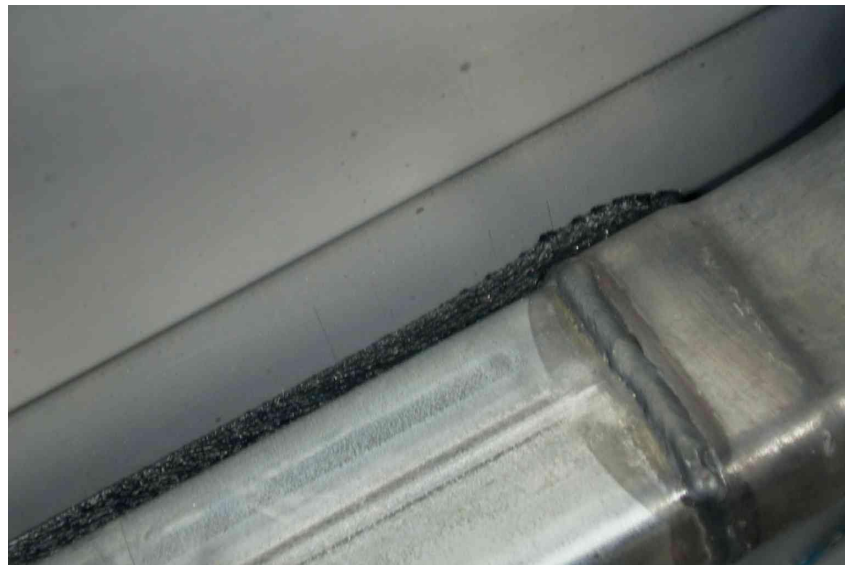
Figure 9.1.4-3 Terostat 3211™ sealing material between the Front Door Lower Tube and the Front Door Outer
