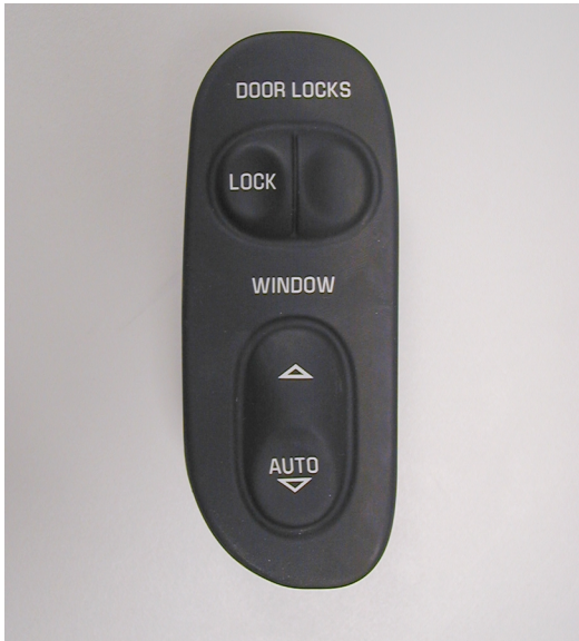
Figure 3.1.1.5.2-3 Front door switch assembly
